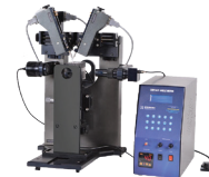
Contact Angle Meter with Dispenser to camera positioning unit, Motorized Substrate Holder, Automated Dispenser, Temperature Control and high speed Camera
