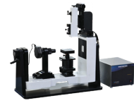
Contact Angle Meter with Dispenser to camera positioning unit, Motorized Substrate Holder, Automated Dispenser, Temperature Control and high speed Camera
