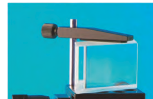
Optics is held by rubber padded clamp
